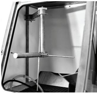
A front loading swing door (with safety lock) allows the operator easy access to the swing arm jig to assist with loading and unloading, the jig features a 48mm shaft over which a wheel can be located, the back of the wheel rests up against x4 round bars and is free to rotate around the central shaft which inclines backwards.
